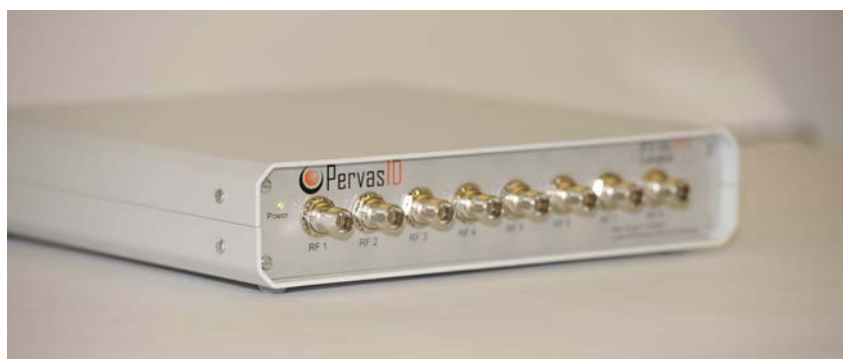
Figure 14: A fixed passive UHF reader
