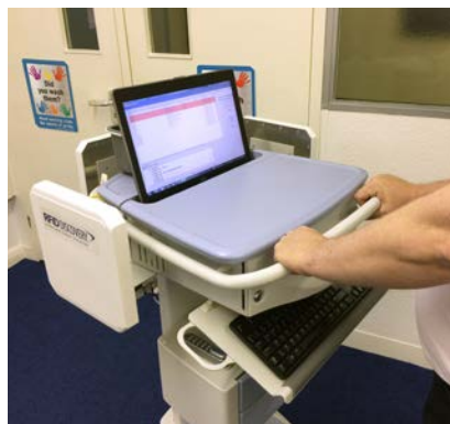
Figure 13: A trolley-based passive reader
