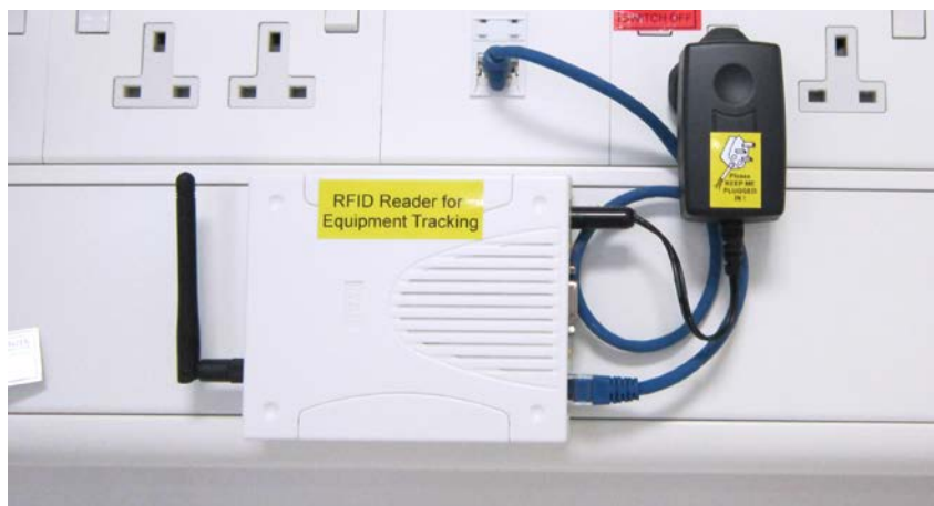
Figure 7: An example of a fixed proprietary active RFID reader
