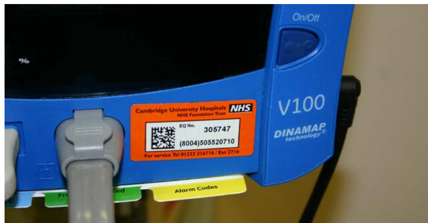
Figure 5: A GS1 barcode on a medical device
