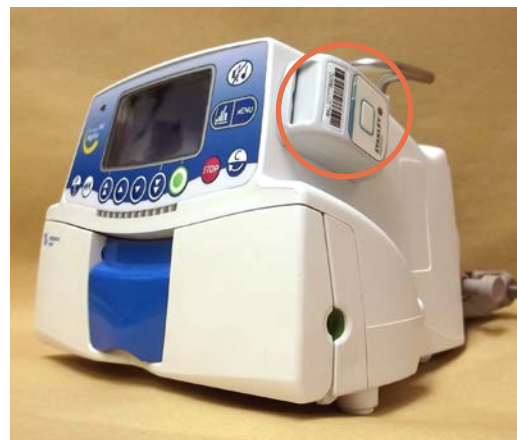
An active Wi-Fi based RFID tag on a medical device
