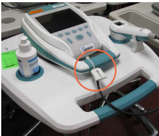
An active non-Wi-Fi based RFID tag on a medical device
