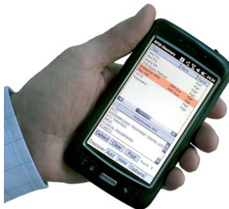
Figure 8: An example of a handheld active RFID reader
